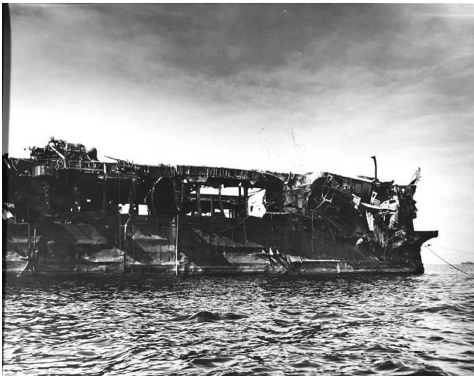
Fig. 4 Damage to USS Independence , documented after Operation Crossroads (US National Archives)
