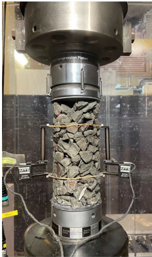
Fig. 7 A picture of an experimental CGM sample under uniaxial loading by MTS machine. The extensometers are connected to the sample to record the strain accurately
