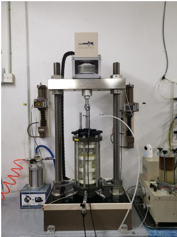
Fig. 3 GDS enterprise-level dynamic triaxial testing system utilized for the cyclic triaxial test
