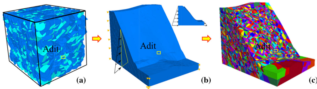
Fig. 14 a Simplified DFN model of the rock slope, b 3D model of the right bank, and c 3D geomechanical model of the right bank
