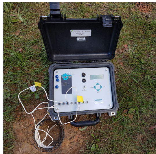
Fig. 6 In situ soil suction measurement
