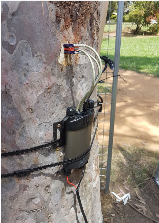
Fig. 7 SFM1 for sap flow rate monitoring
