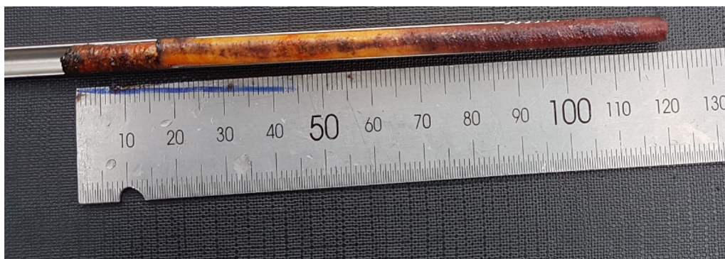
Fig. 8 Sapwood estimate by applying an indicator dye
