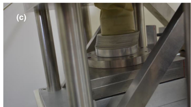
Fig. 2 View of NGI type DSS setup: a general view of the apparatus; b schematic illustration of soil specimen in DSS cell; c a sheared specimen
