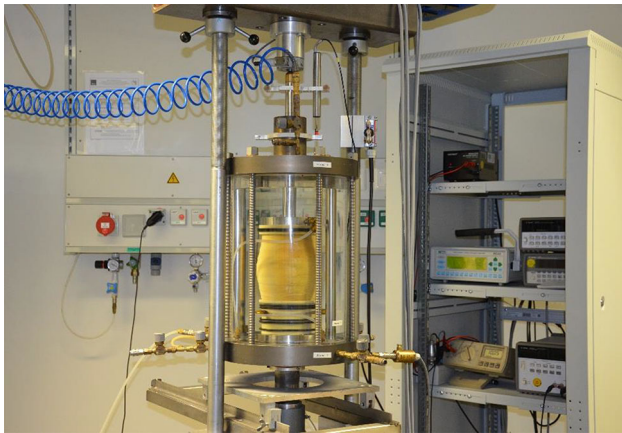
Fig. 3 Triaxial device applied for the current experiments
