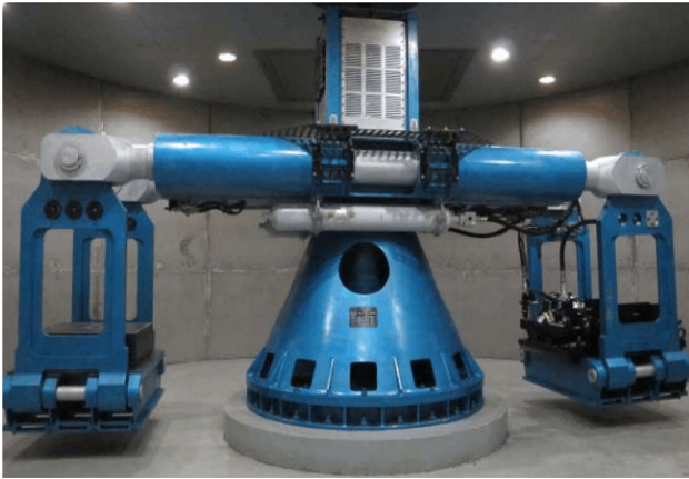
Fig. 4 Photograph of ZJU-400 geotechnical centrifuge
