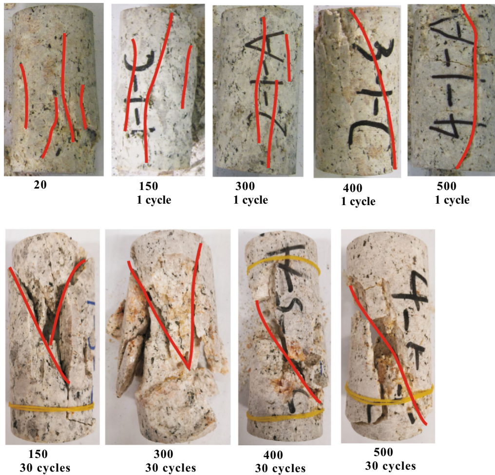
Fig. 9 Macrofractures of granite after heating and water-cooling treatment for 1 and 30 cycles
