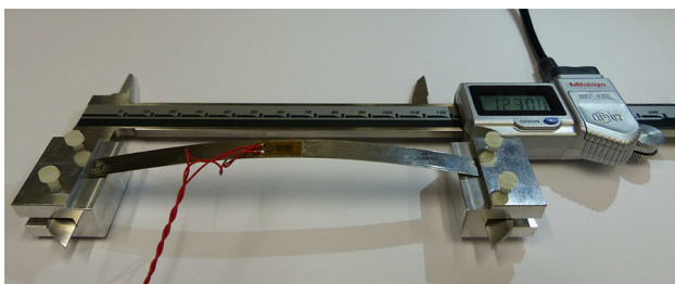
Fig. 5 Calibration of an LDT by controlled application of a bending induced by horizontal displacement of one end of the LDT
