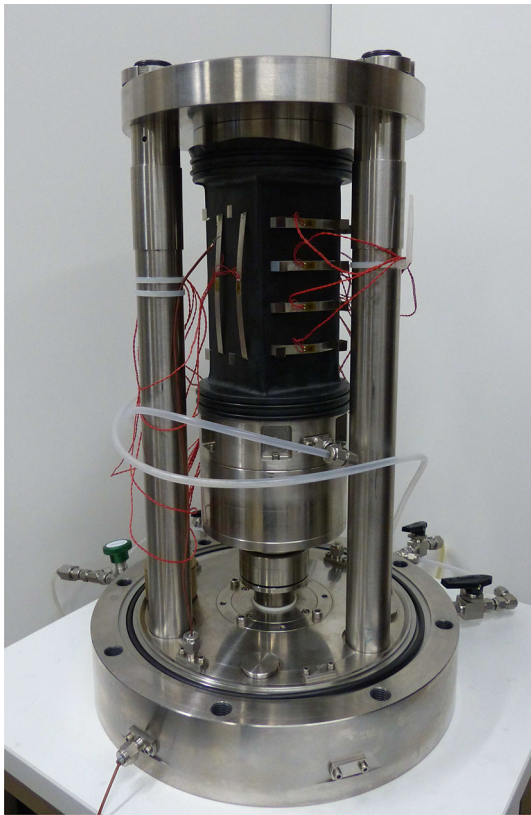
Fig. 4 Photograph of a sample equipped with LDTs
