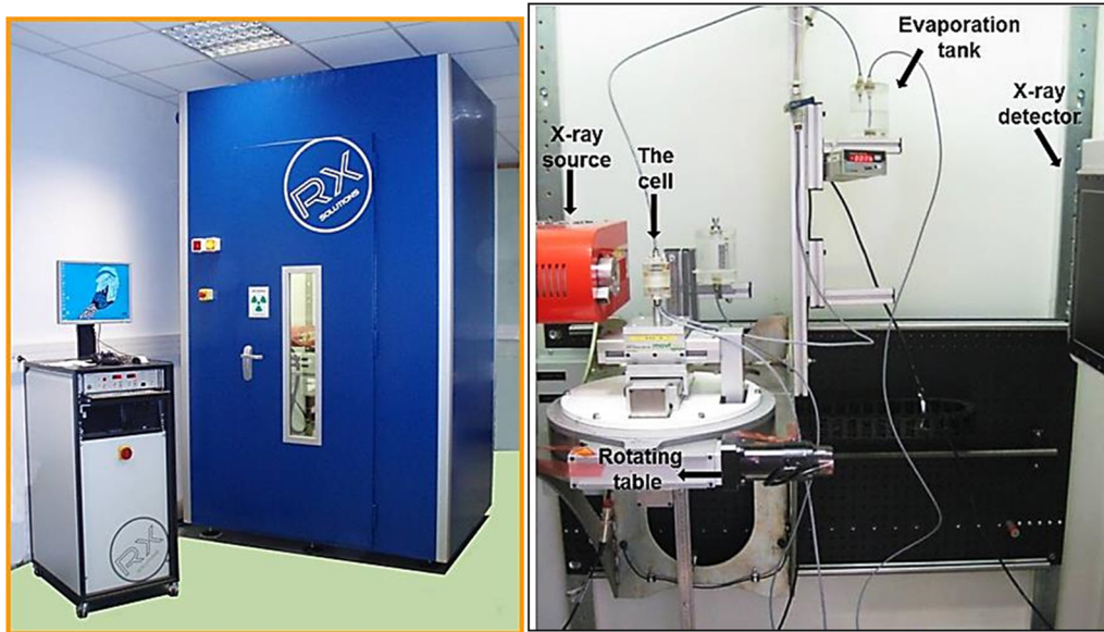
Fig. 6 X-ray tomograph in Laboratoire 3SR: (left) a picture of the cabin, (right) the inside of the cabin with the micro-retention cell in place
