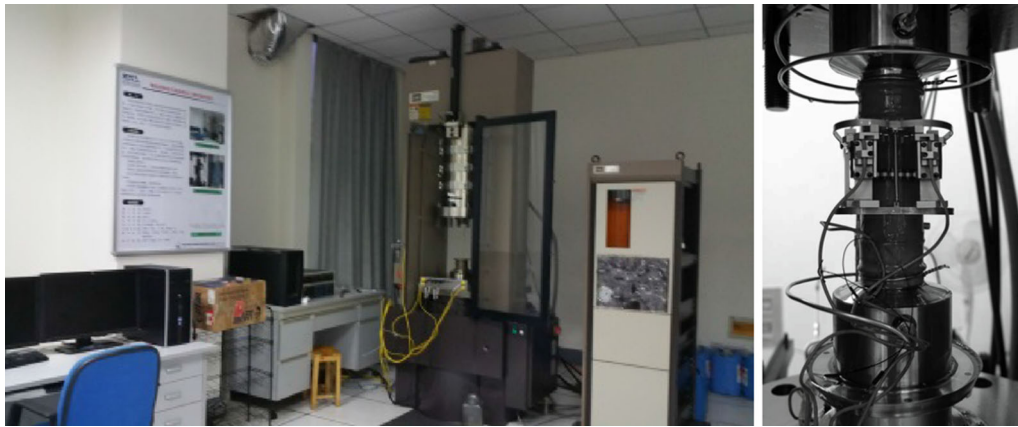
Fig. 6 MTS815 Flex Test GT and PCI-II acoustic emission system used to test carbonaceous slate samples
