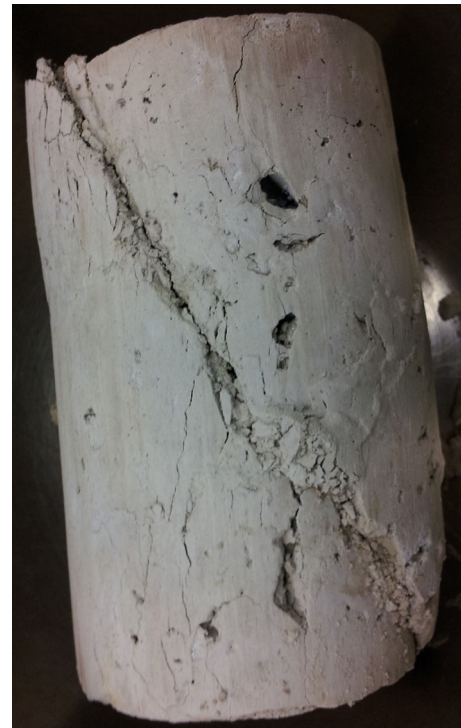
Fig. 9 Typical modes of deformation of improved triaxial CIUC specimens following testing
