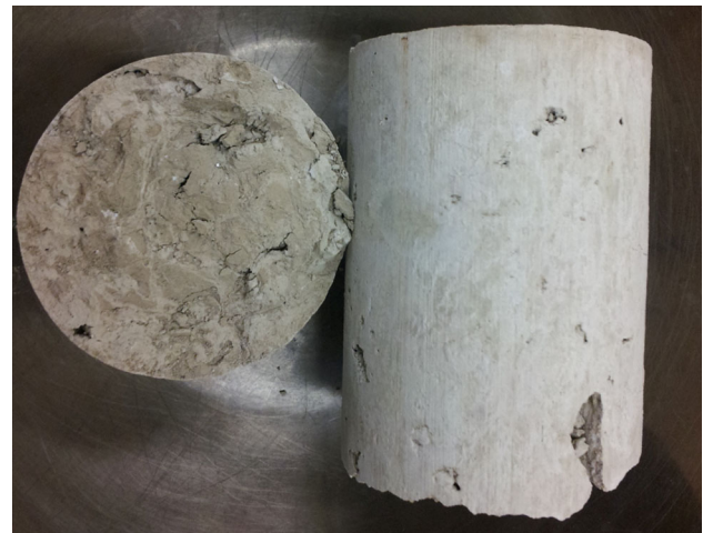
Fig. 10 Typical modes of deformation of improved triaxial CIUE specimens following testing
