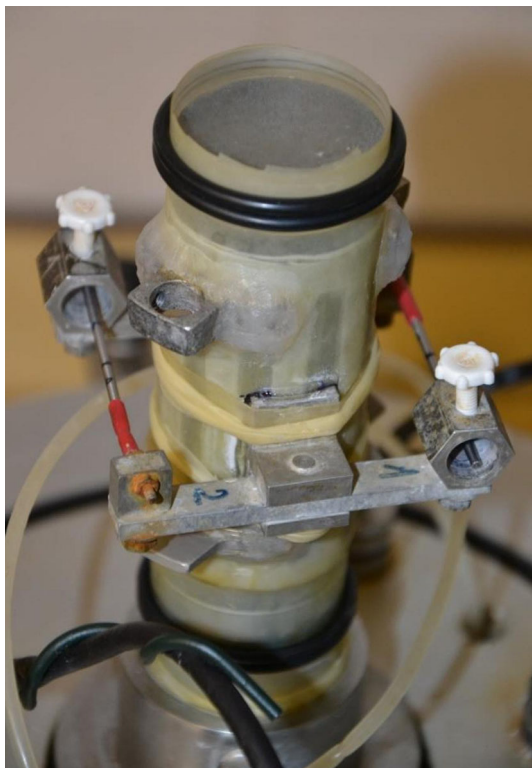
Fig. 8 Setup for local LVDT measurements of radial and axial strain (LVDTs not mounted for clarity of the photograph)
