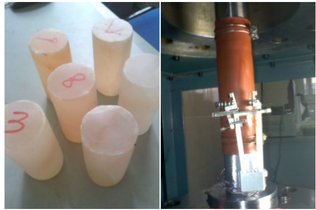
Fig. 1 Manufactured salt sample and installation method
