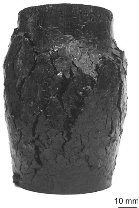
Fig. 6 Picture of a asphalt concrete specimen after failure
