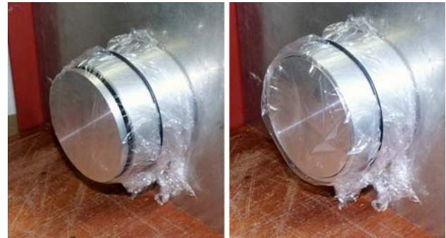
Fig. 17 Model tunnel with cling foil protection against sand ingress
