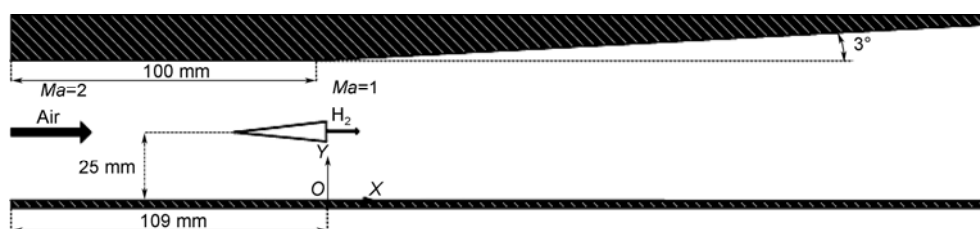
Figure 1 A schematic of a typical strut-based scramjet combustor.
