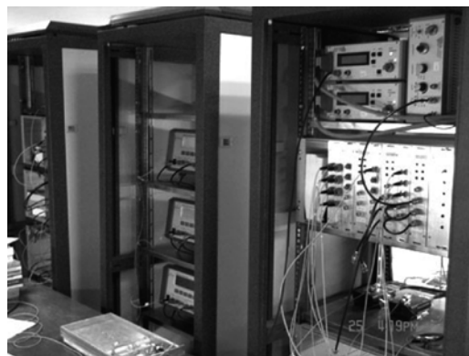
Figure 4 Practical QKD system. Each part of the system was compacted into a 5U-height (225 mm) rack mounts without temperature controller.
