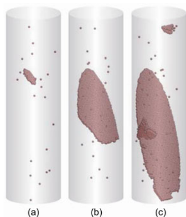
Figure 9 (Color online) Initial yielding deformation of the defect-free Cu nanowires. At the elastic limit (a), a dislocation nucleates at the surface and emits across the nanowire section (b), and finally absorbed by the surface (c). HCP atoms are shown in red in this figure and following figures.
