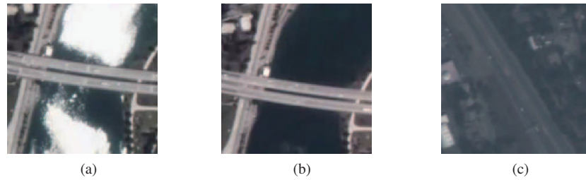
Figure 2 (Color online) Low imaging quality in satellite videos. (a) Overexposure in a bridge scene; (b) a reference frame of (a) without overexposure; (c) low contrast in a highway scene.
