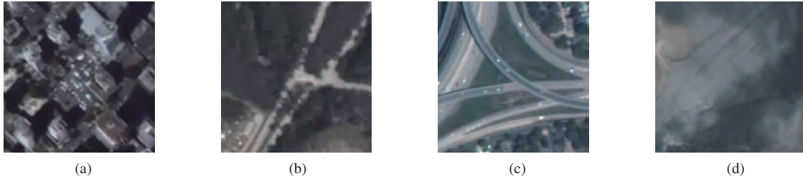
Figure 1 (Color online) Various occlusion phenomena in satellite videos. (a) Moving targets are occluded by the shadow of high buildings in a parking lot scene; (b) a highway scene is occluded by dense trees; (c) moving targets are occluded when they pass through the bottom of the overpass; (d) a highway scene is occluded by thin clouds.
