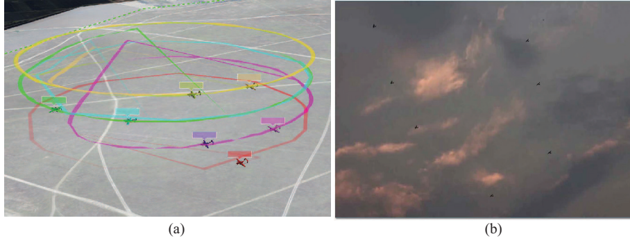
Figure 5 (Color online) Seven UAVs circling in an ordered alignment. (a) Achieving alignment in the ground station; (b) the achieved alignment in the field experiment.
