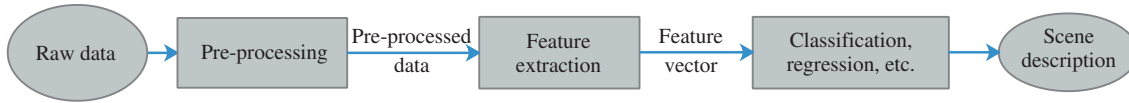
Figure 8 Cognitive process of understanding traffic scenes. It is made up of pre-processing, feature extraction, post-processing such as classification, regression steps and finally obtains the description of the scene.
