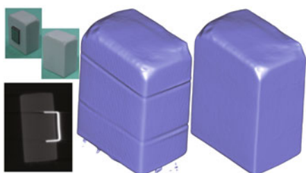
Figure 9 A demonstration of robustness of our method to CT scanning artifacts. Left: photos of front- and back-side of an eraser with a staple (top) and a cross-section of the CT scanning (bottom). Middle: the back-side face of the eraser obtained with isosurfacing. Right: the face obtained with interpolating the edge-points.
