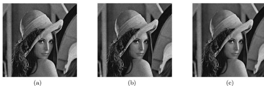
Figure 4 Comparison of Trilateral Filter and MNF (3). (a) The noisy image e ( \sigma = 10 ); (b) Image e restored by Trilateral, PSNR=33.23*(33.23); (c) Image e restored by MNF, PSNR= 34.86.
