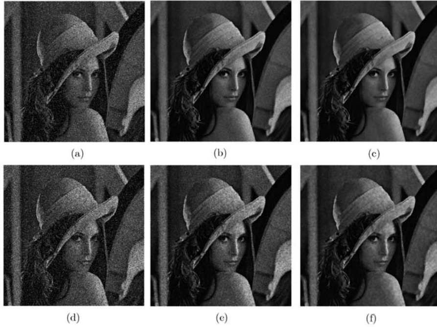
Figure 2 Comparison between trilateral filter and MNF (1). (a) The noisy image a ( \sigma = 10, p = 0.2 ); (b) Image a restored by Trilateral, PSNR=31.79; (c) Image a restored by MNF, PSNR=32.84; (d) the noisy image b ( \sigma = 20, p = 0.2 ); (e) Image b restored by Trilateral, PSNR=27.73; (f) Image b restored by MNF, PSNR=30.23.
