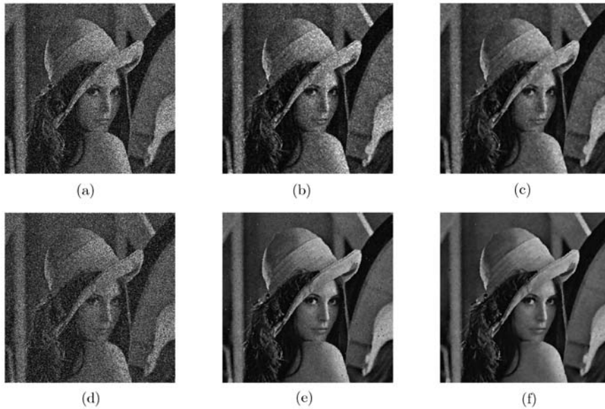
Figure 3 Comparison between trilateral filter and MNF (2). (a) The noisy image c ( \sigma = 30, p = 0.2 ); (b) Image c restored by Trilateral, PSNR=24.92; (c) Image c restored by MNF, PSNR=27.33**; (d) the noisy image d ( \sigma = 10, p = 0.4 ); (e) Image d restored by Trilateral, PSNR=28.75; (f) Image d restored by MNF, PSNR=29.96.
