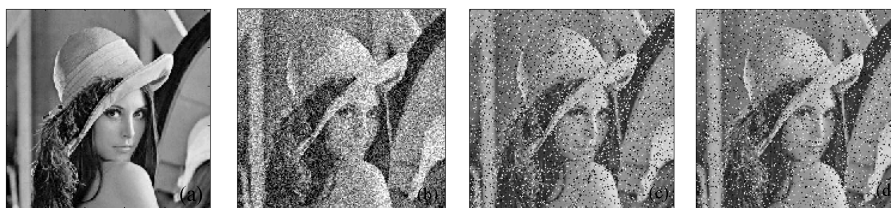
Figure 6 Decrypted images when the cipher-image is blurred by noise or geometrical distortion (four rounds of encryption). (a) Noise free; (b) gauss noise ( \mu=0 , \sigma=10 ); (c) scratching with vertical 5% pixels rubbed; (d) Salt and pepper noise ( p=0.05 ).
