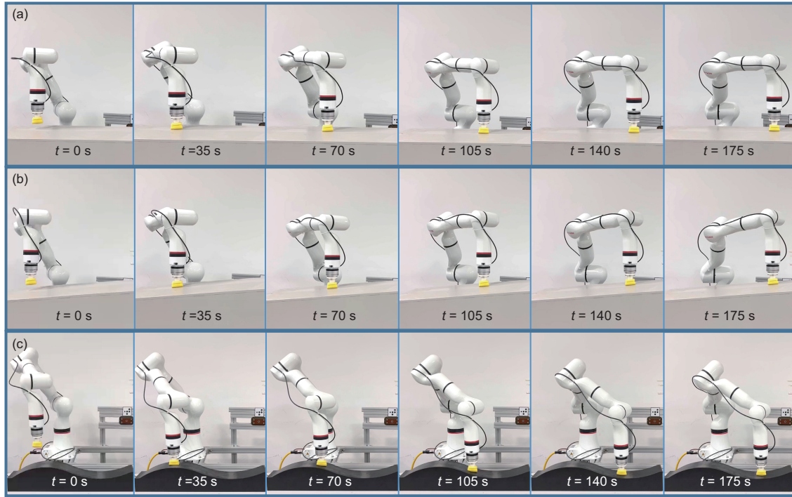
Figure 9 (Color online) Case studies using a different robot: (a) the flat surface, (b) the slope surface, and (c) the curved surface.
