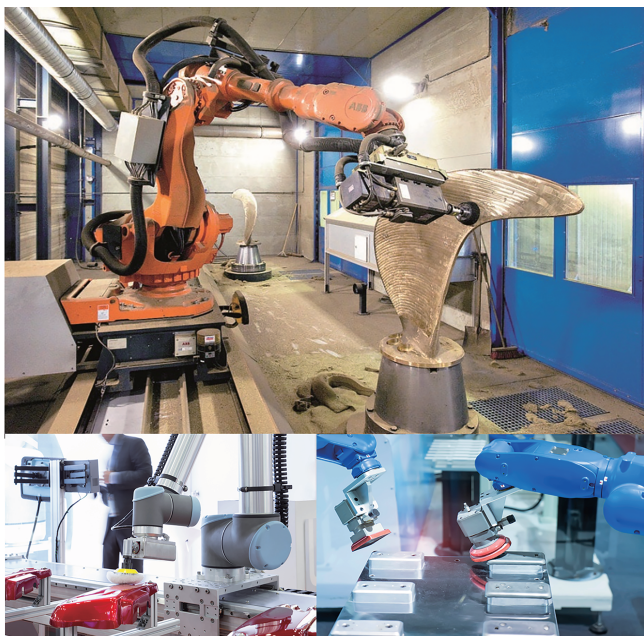
Figure 1 (Color online) Typical robotic polishing and grinding tasks [2].
