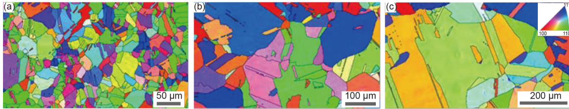
Figure 1 (Color online) Grain orientation maps obtained by electron backscattering diffraction for annealed coarse-grained Cu with different average grain sizes for DPD treatment. (a) 30 \mu\text{m} ; (b) 150 \mu\text{m} ; (c) 540 \mu\text{m} .
