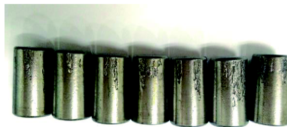
Figure 2 (Color Online) Fatigue damage on the test roller surface.
