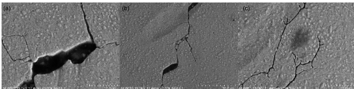
Figure 8 The micro appearance of the subsurface crack in Figure 6(b).
