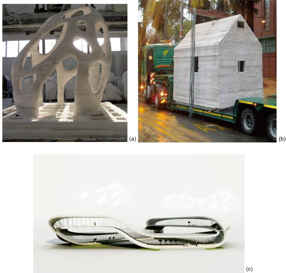
Figure 3 (Color online) Large-scale structures manufactured via D-shape technology. (a) 1.6 m high sculpture; (b) a complete house printed in one single process; (c) landscape house design based on a Möbius strip.
