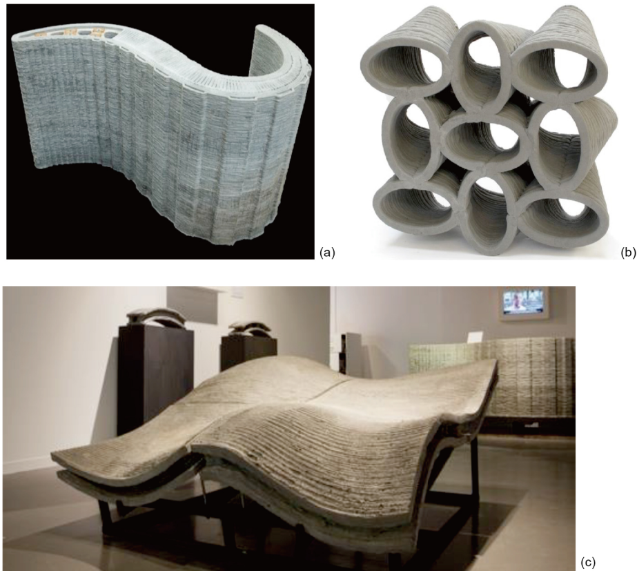
Figure 7 (Color online) 3D components manufactured by concrete printing. (a) Wonder bench (2 m×0.9 m×0.8 m); (b) acoustic damping wall element; (c) curved-layered construction component.
