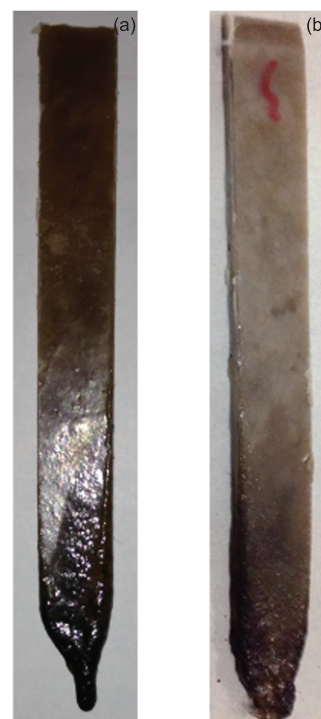
Figure 9 (Color online) Digital photos of the specimens after vertical burning test. (a) Jute/PLA/7DOPO; (b) jute/PLA/7DOPO-ICN.
