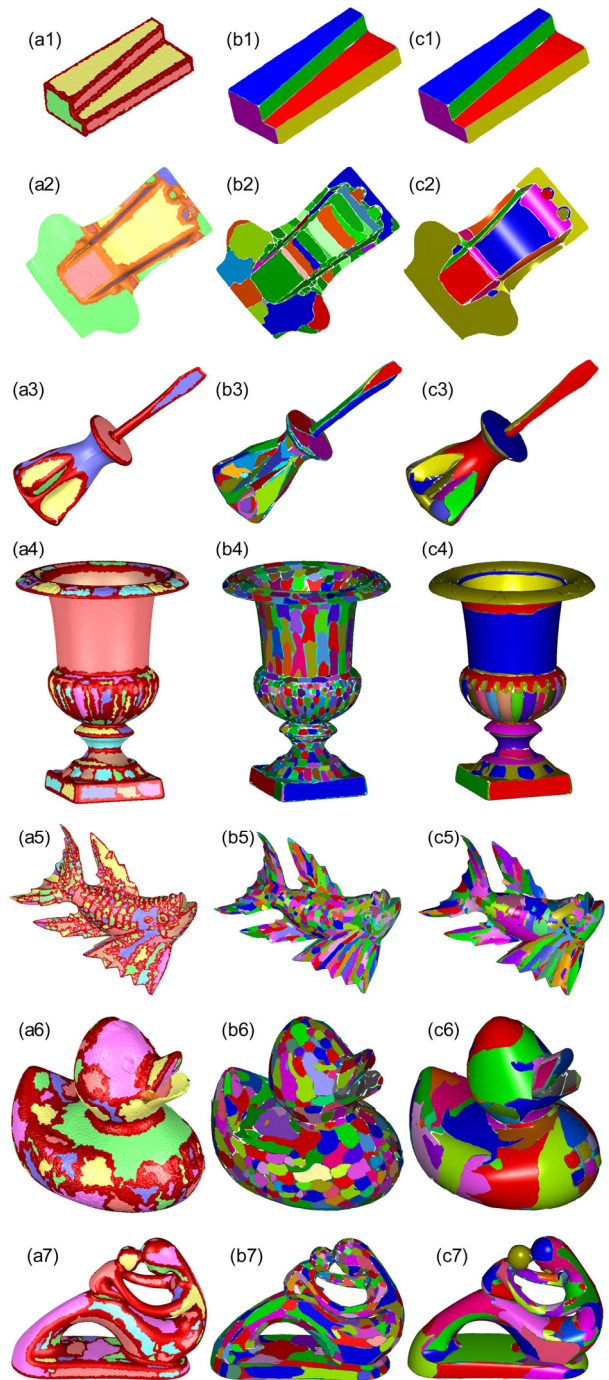
Figure 8 (Color online) Segmentation results of the box, the sheet metal part, the screwdriver, the vase, the fish, the duck, and the statue: (a1)–(a7) are from Geomagic Studio; (b1)–(b7) are from our planar segmentation; (c1)–(c7) are from our quadric segmentation.
