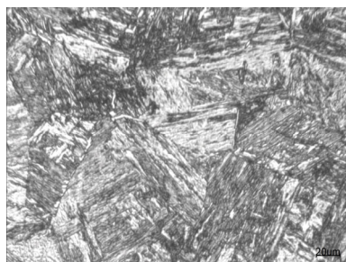
Figure 9 Optical micrograph of the cylindrical blank after austenitized at 910°C for 10 min and cooled in 5% NaCl solution.
