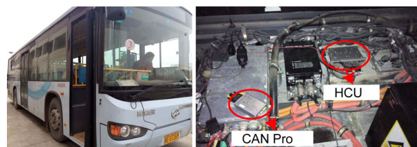
Figure 9 (Color online) The tested bus and devices.
