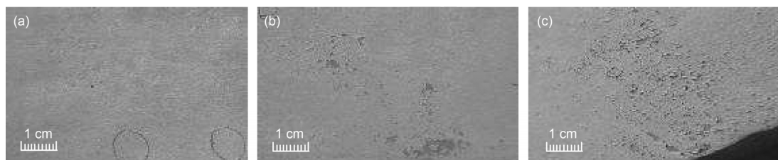
Figure 4 Macroscopic appearance of samples sprayed (a) three times, (b) five times, and (c) seven times.
