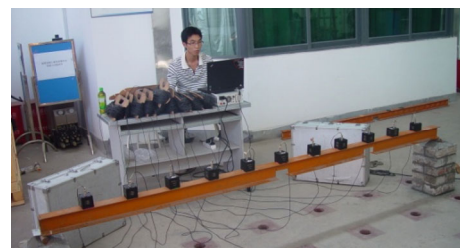
Figure 4 (Color online) Ambient vibration test of the steel beam model.
