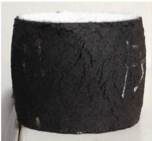
Figure 2 (Color online) Failure model of the CA mortar layer.
