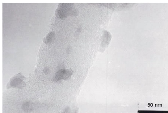
Figure 8 TEM image of ZnO decorated CNTs; CNTs were treated only by acid modification.
