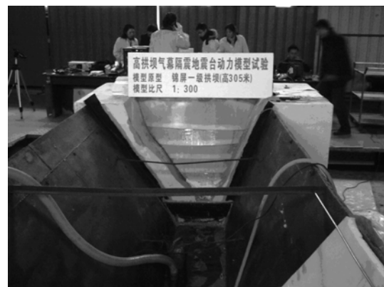
Figure 12 Photo of the experiment model on the shaking table.
