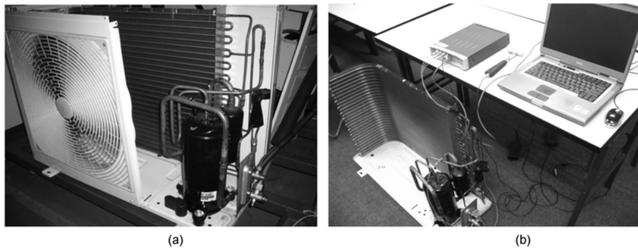
Figure 3 (a) Suction and discharge tubes in air conditioner outdoor unit mounting to their adjacent parts; (b) equipments setup of modal impact hammer test.
