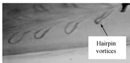
Figure 11 The flow structures produced by the circular ZNMF jet in cross flow, the actuator orifice is at the top of the image, and the flow direction is from right to left [24] .
