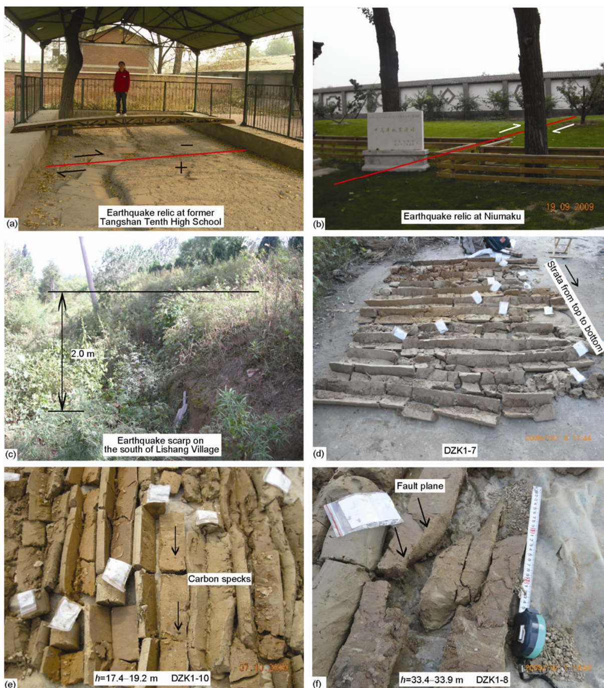
Figure 2 Earthquake relics and cores recovered from boreholes photos at Niumaku. (a) Earthquake relic at former Tangshan Tenth High School. The surface rupture offset a trail right-laterally, west side up, camera to east. (b) Earthquake relic at Niumaku on Kangbai Road in Tangshan. The tree line is twisted by the rupture zone, west side up, camera to north. (c) Earthquake scarp south of Lishang village in Tangshan, camera to NE. (d) Core array from borehole DZK1-7 at Niumaku. The strata are mainly yellow and yellowish gray in color; the ratio of loam and sandy loam to silty sand is 1:1. (e) Core samples from depths of 17–19.2 m in borehole DZK1-10 at Niumaku. The loam contains carbon specks. On the right is silty sand. (f) A straight fault plane dipping 75° appears in the brown clay at depths of 33.4–33.9 m in borehole DZK1-8 at Niumaku; there is a thin layer of sand on the fault plane.
