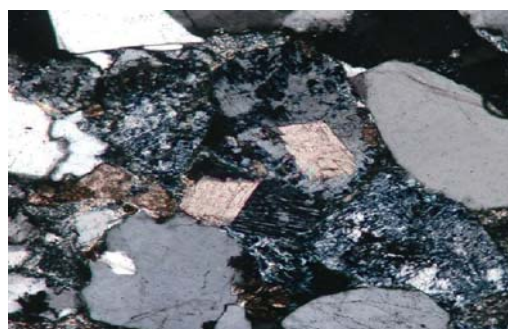
Figure 7 Ferro dolomites alternated feldspars. Well Qiongxi 13-1 (2450.87 m, cross-polarized light, ×100).
