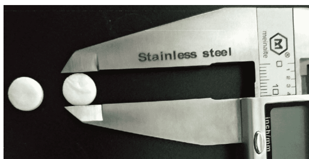
Figure 5 Optical image illustrating the PCL scaffold prepared by supercritical foaming process.
