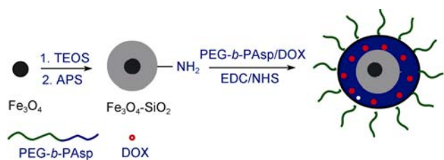
Figure 1 Synthesis of multilayer and multifunctional hybrid nanoparticles and the process of drug loading.
