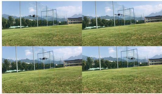
Figure 11 The gap traversal of the quadrotor along a safe path
