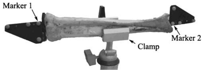
Fig. 1. Tibia–fibula specimen with marker plates attached and mounted in the clamp. Markers 1 and 2 were positioned to define the long axis of the tibia. The markers on each plate were used to define local coordinate systems from which the relative rotations were determined
