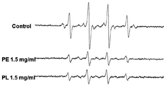
Fig. 2 Hydroxyl radical scavenging activities of ethanol and ethyl acetate extracts from root powder of extract derived from Polygonum cuspidatum . The signal intensities of DMPO–OH adduct were determined by electron spin resonance spectrometry and recorded 8 min after reaction initiation in phosphate-buffered solution (pH 7.4) containing 100 mM DMPO and the following reactants: Control (4% ethanol), 1.5 mg/ml of ethanol extract (PE), ethyl acetate (lipophilic levels) extract (PL)
