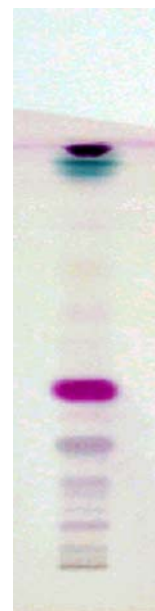
Fig. 1 Detection of terpenoids on thin-layer chromatography (TLC) using anisaldehyde sulfuric acid reagent
