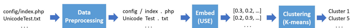
Fig. 1 The semantic clustering process used to group similar words. Each word in the wordlist is encoded by using the Universal Sentence Encoding (USE), then K-means clustering is used to group similar words
